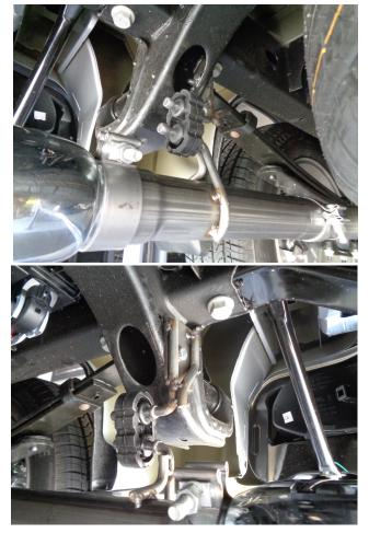
Step 5. As this vehicle was not setup for dual exhaust from the factory, hanger brackets will need to be installed. Install the hanger brackets on the rear frame section using the supplied fastener hardware as shown
